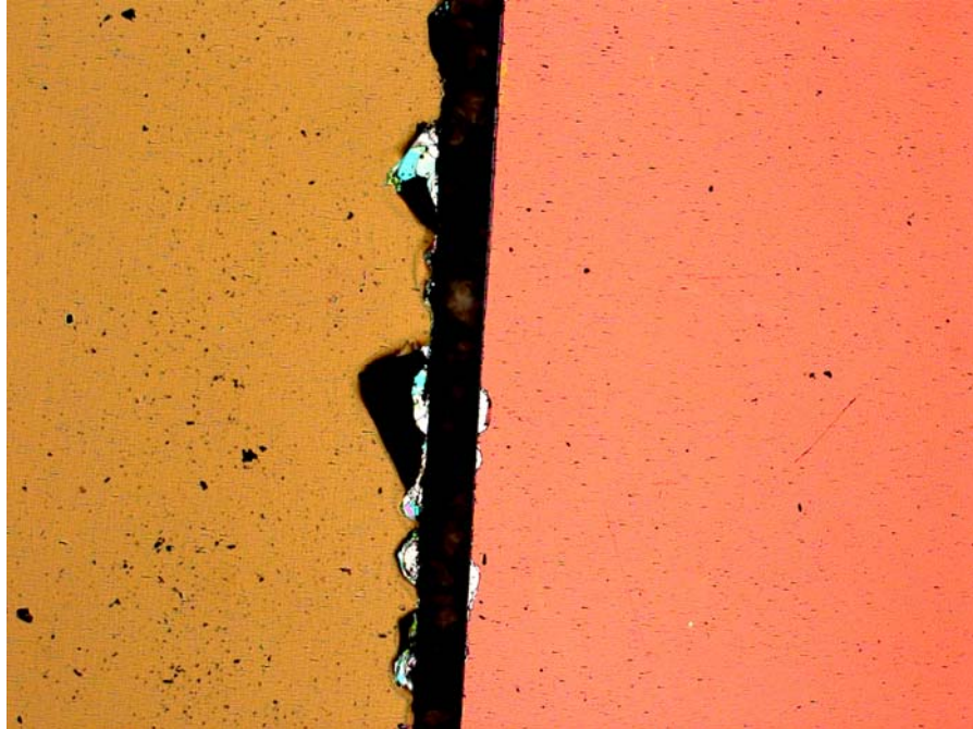
Figure 11. Edge Comparison of a Scribed/Cleaved and a Diced Tandem Filter (50X Magnification)
